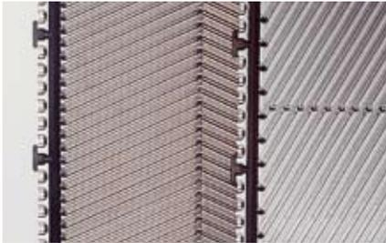
**4. Reassembly with used glue-free gaskets**
