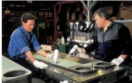
**5. Re-gluing of glued gaskets**
